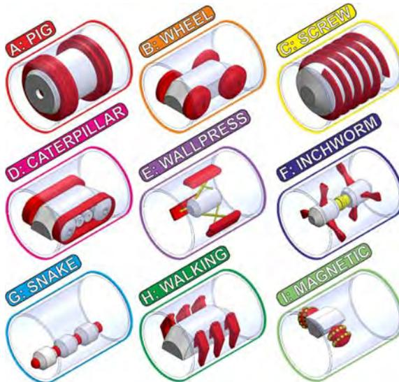
Figure 1: Basic in-pipe robotic locomotion types A – I.
